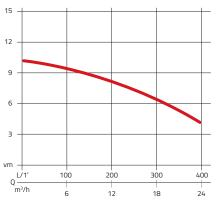
The diagram shows you the pumping capacity of the Rössle submersible pump MEGA in m<sup>3</sup> per hour in relation to the pumping height.
