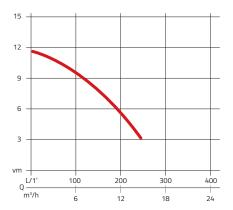
The diagram shows you the pumping capacity of the Rössle submersible pump KILO in m³ per hour in relation to the pumping height.
