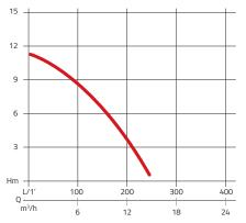
The diagram shows you the pumping capacity of the Rössle submersible pump FLAT-ROSS in m<sup>3</sup> per hour in relation to the pumping height.
